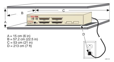
Figure 3-1 Tabletop or Shelf Installation
